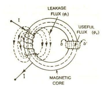
Most of the flux is set up in the core of the solenoid and passes through the particular path that is through the air gap and is utilised in the magnetic circuit. This flux is known as **Useful flux**  $\phi_u$ .
